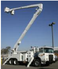
Carmenita delivers natural gas trucks like this CNG Autocar with Altec aerial rig and fuel system by AFV Fab
